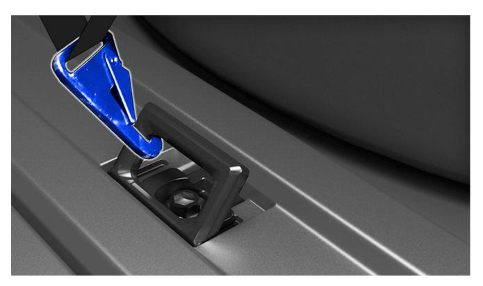
4. Connect the strap, then tighten starting from the RH side using the slack adjuster. Secure the excess strap to the top of the cover with the Velcro.
